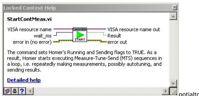
**DDE Server.** DDE Server is a functionality within the *HomSoft* Windows SW hence it needs the *HomSoft* Windows visualization and control software option, too. The DDE Server enables another (customer's) Windows program to extract measurement results from *HomSoft* program, e.g. to a LabVIEW environment.
