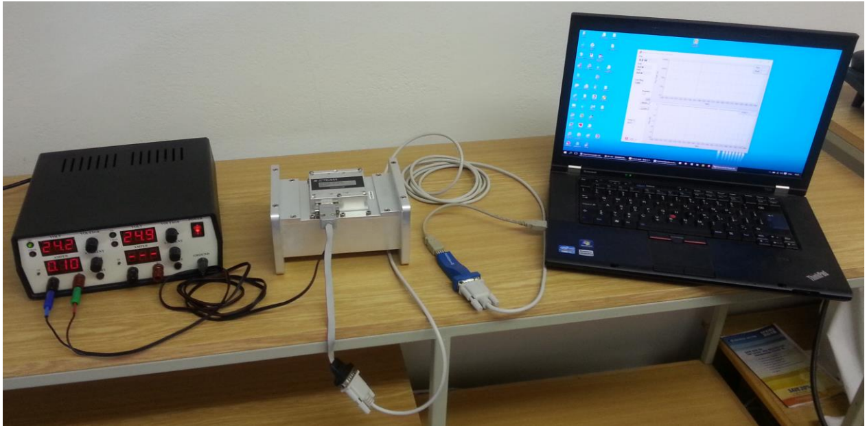
Fig. 17. Illustration of BPM – PC connection (Model BPM112 shown).
